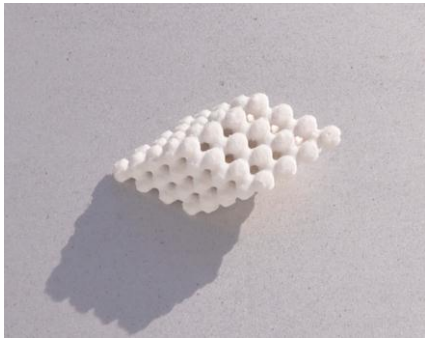
Fig. 3: Diamond structure made out of piezo ceramic
