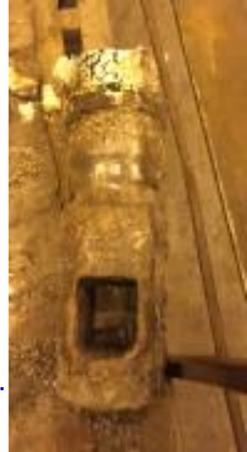
Pic:3 Used piece after 7 heats
