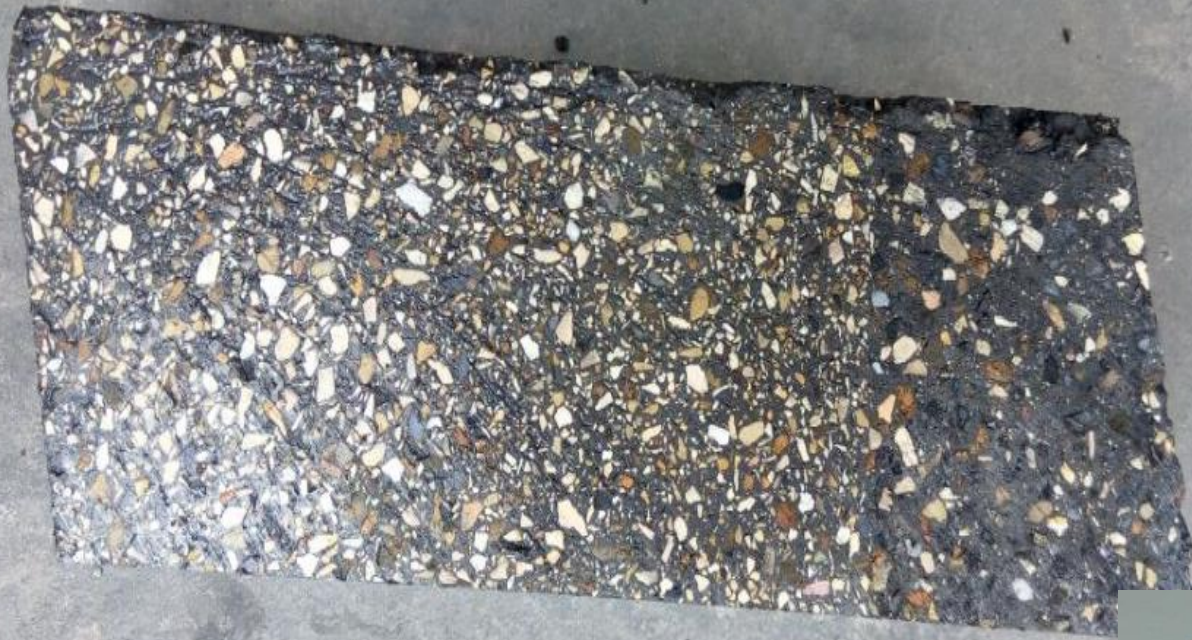
Two-layer brick for hot metal ladle lining
