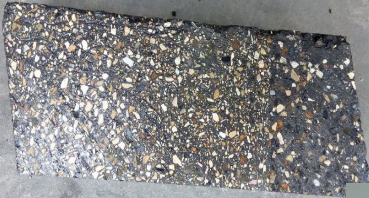
Two-layer brick for hot metal ladle lining
